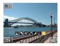
Hold the camera steady and aim at the subject. The camera will automatically choose the appropriate mode to suit the lighting conditions of the scene you are photographing.
